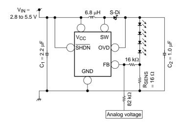
3) Input PWM signal with filtering to FB terminal
