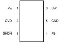
Note 1: This IC could be destroyed in some case if amounted in 180° inverse direction. Please be careful about IC direction in mounting.
